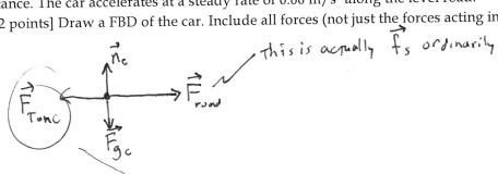
b) [2 points] Draw a FBD of the truck. Include all forces (not just the forces acting in the horizontal direction).
