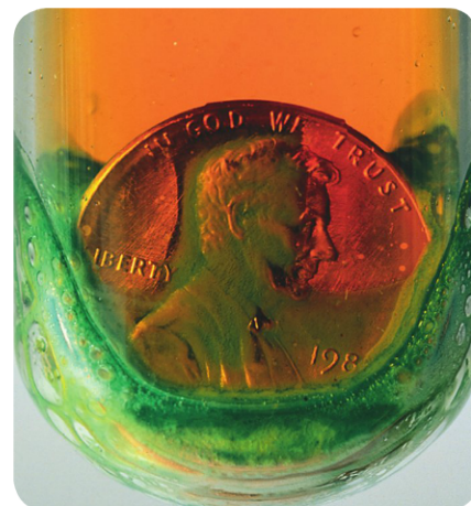
▲ Copper metal reacts with nitric acid (HNO 3 ) to yield the brown gas NO 2 .
