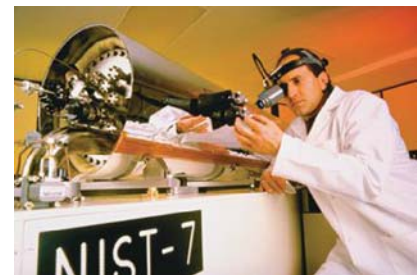
An atomic clock at the National Institute of Standards and Technology is the primary standard of time.
